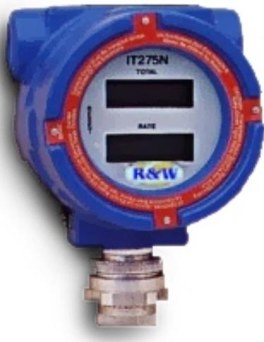
provides flow totalization and rate in most engineering units. Total and rate are displayed via two 8-digit liquid crystal displays. The totalizer reset function is accomplished externally by a magnetic field to retain unit integrity while permitting complete operational control in hazardous environments. In addition, the IT275 provides an analog 4-20mA output. The 4-20mA loop control extracts no power from the loop.
